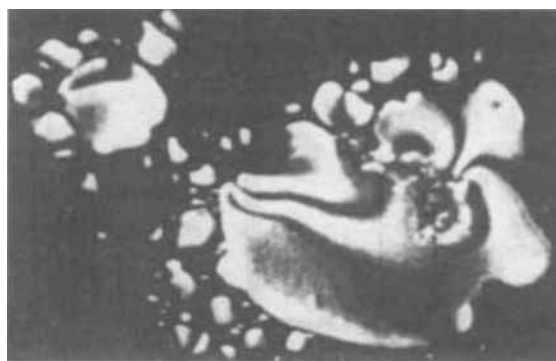
FIGURE 6 Polarizing optical micrograph of PPCH504T; Schlieren texture at 124 °C in the cooling process.
